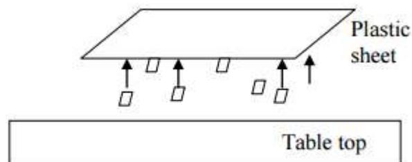
The negatively charged plastic sheet repels the electrons in the tissue bits, pushing them lower.
